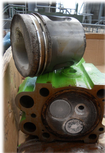
Silicon deposits on a head & valves causing a collision between valves and piston crown
