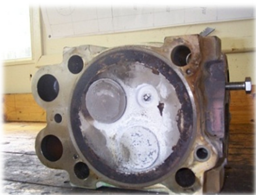
Silicon deposits on a head & valves causing a collision between valves and piston crown
