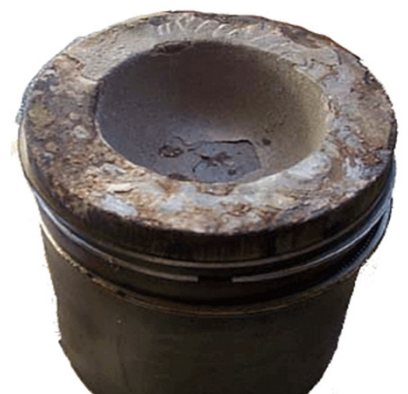
A piston coated in deposits
